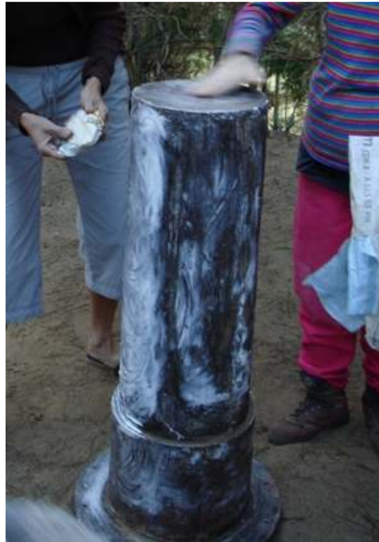
Grease the inner core with cooking fat, paying attention especially to the diffuser plate ledge.
