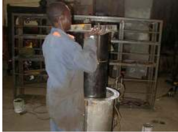
Lower the inner core carefully into the outer shell.
